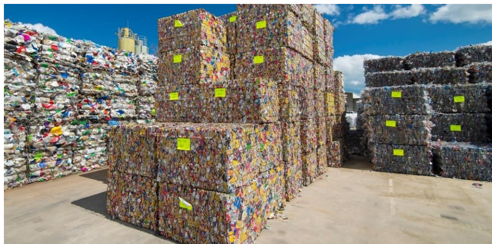
In the stacks from left to right are coloured HDPE plastic, aluminium cans and PET plastic.
